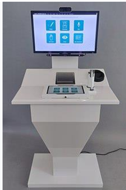
Biometric Island examining facial image 2D and 3D, voice timbre, and verifying handwritten signature
